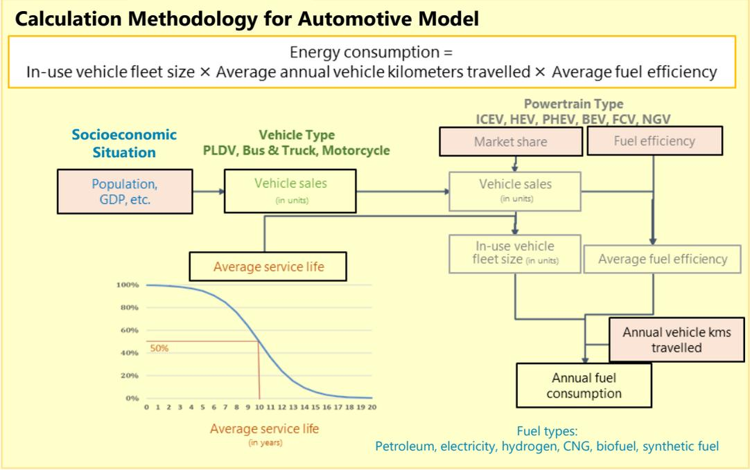
Figures for future fuel consumption (CO2 emissions) were calculated using IEEJ's macroeconomic model and energy demand model reflecting JAMA's powertrain mix estimates.
