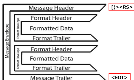
図 B-1 Enveloping Structure
