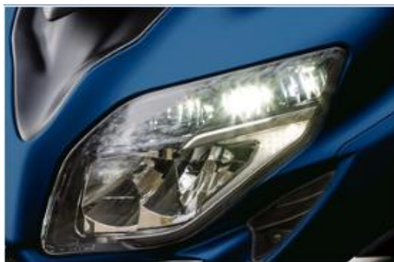
Activation of additional lighting units to illuminate the bending road
